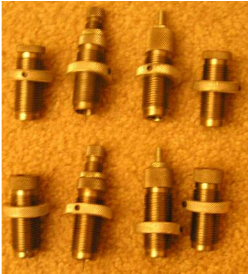
This is a comparison of a 1972 RCBS set to a 1975/76 RCBS set. Note the different knurling height on the die sets (no effect on functionality). The dies are pictured from L to R: Size, Expand/Decap, Seat, Crimp.
