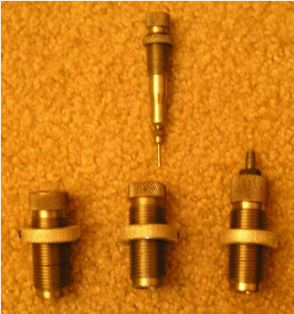
Here's a common 357 AMP Die Set, RCBS Part # 35505, the tapered Autmag cartridges used a 3 die set: Size Die, Expander/Decapper, and Sear/Crimp Die.
