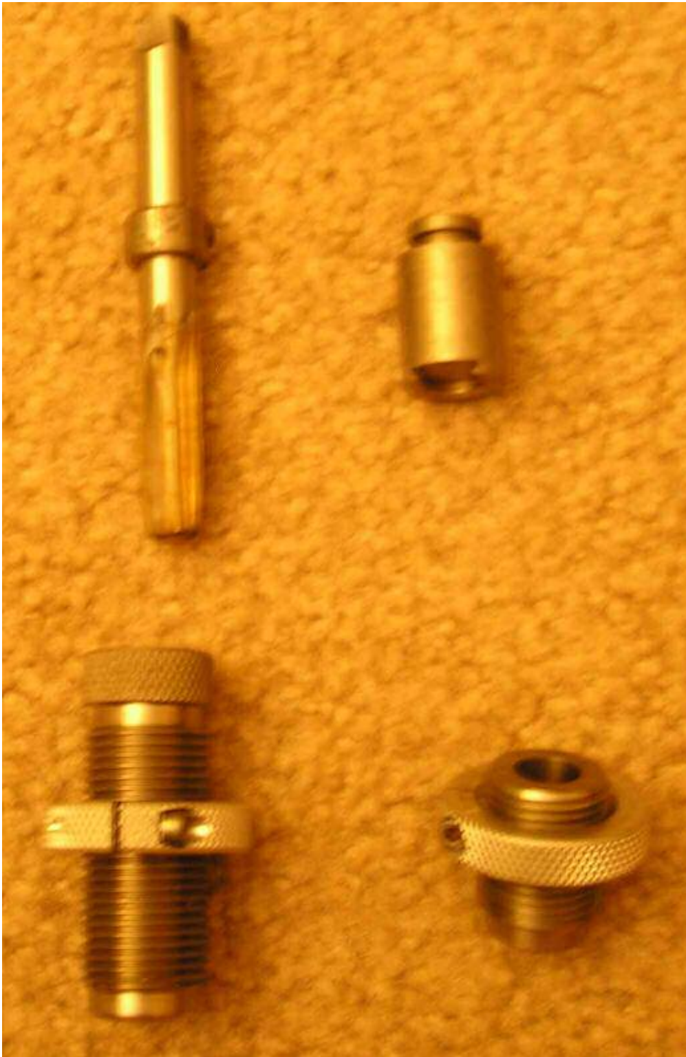
Complete 44 AMP Case forming set, RCBS Part # 40039 (sometimes # 55000 was used). On left, Reamer Die w/ Reamer, on right top, RCBS extended shell holder #3 for case trimming, on right bottom form/trim die. Note Reamer is still in original protective coating.
