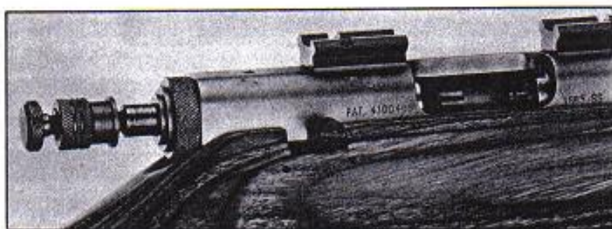
The sliding hammer and its heavy coil spring are retracted by pulling back on the cocking knob until the sear engages. The assembly is retained by the threaded end cap. The side safety blocks the sear and a secondary safety blocks the hammer fall.
