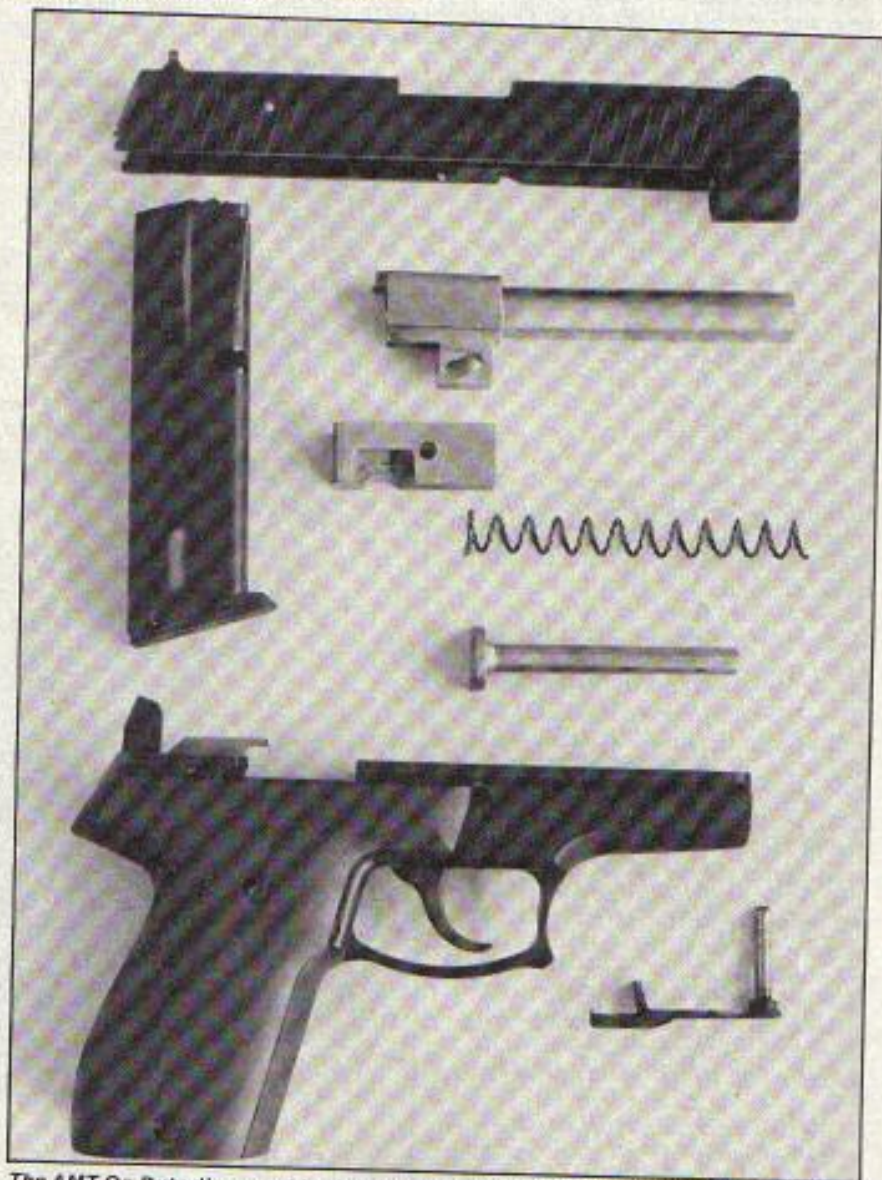
The AMT On Duty disassembles into these eight component parts, with the ejector integrally pinned to the grip frame. The small part to the right of the magazine is the breech block and it also incorporates the extractor, as discussed in the text.
