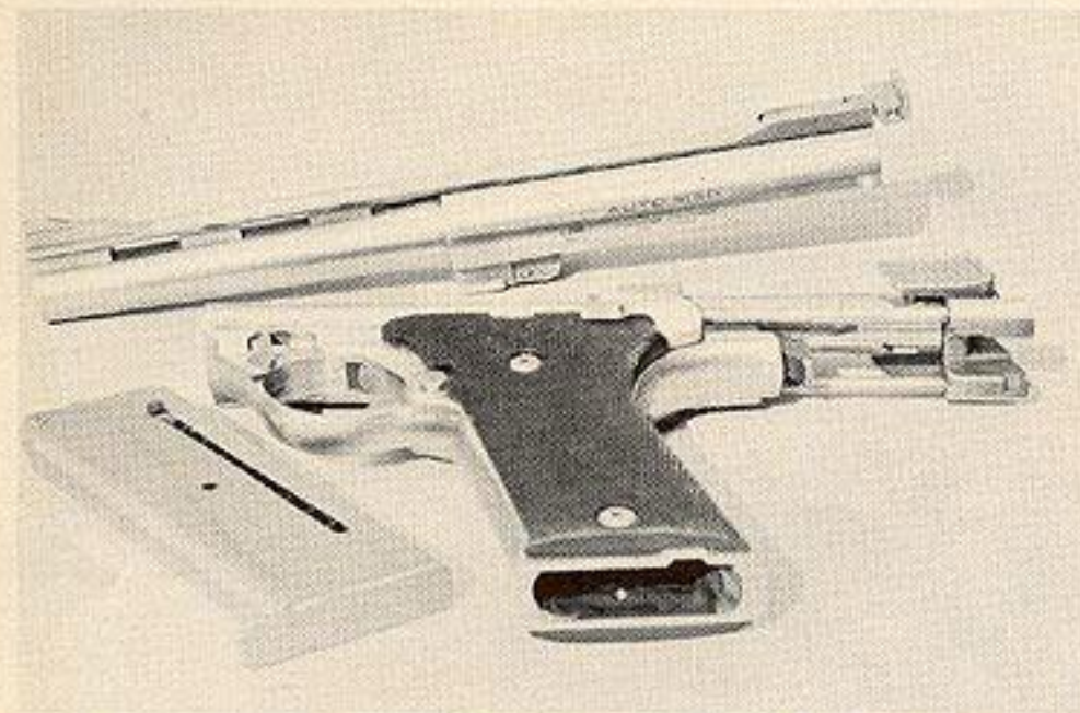
Auto Mag easily field strips into three sub-assemblies. Note that barrel, sights and barrel extension are one integral unit. Stud on magazine follower is to actuate slide hold-open, not an aid in loading.
