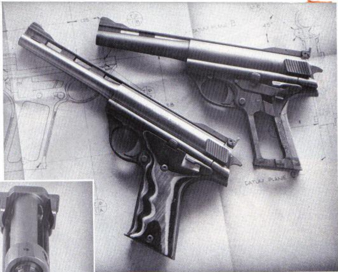
Above: From prototype to L. E. Jurras Custom Model 100. Note barrel and grip change. Left: Bolt seen at front, ready to drive in a round.
