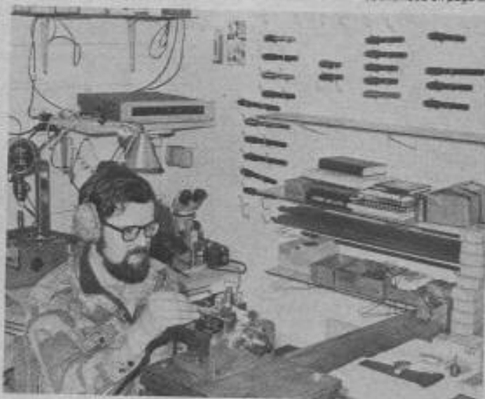
Lumant is one of the niggardly few hand-loader/shooters who have their very own ballistics laboratory set up. Here he prepares to insert copper-crusher cylinder in Phelps-type universal pressure gun. Other pressure barrels are tacked on the wall at rear.
